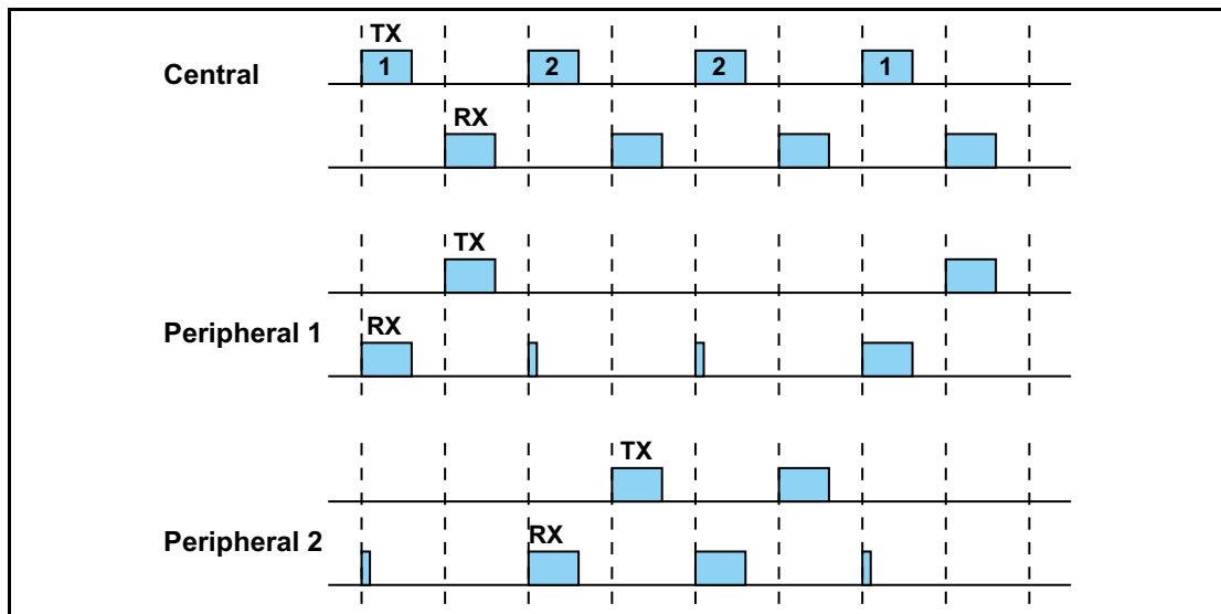
Figure 8.8: RX/TX timing in multi-Peripheral configuration
