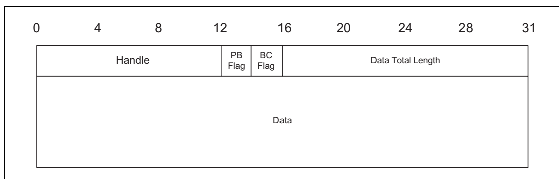
Figure 5.2: HCI ACL Data packet
