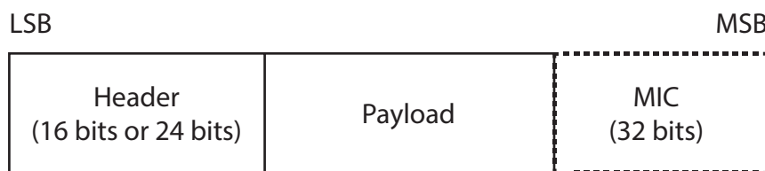
Figure 2.24: Data Physical Channel PDU
