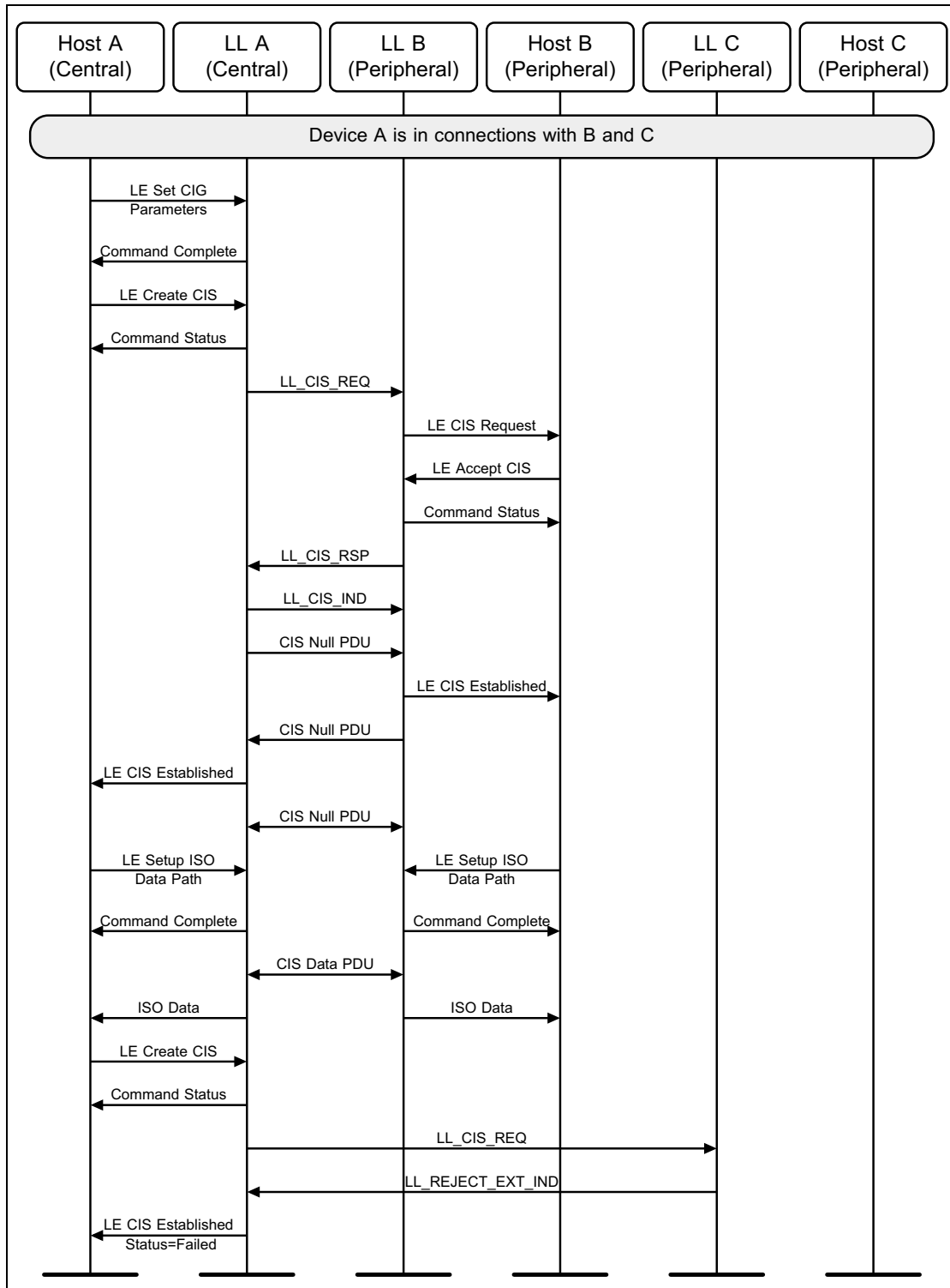
Figure 6.47: The Link Layer in Device C rejects a CIS from Device A
